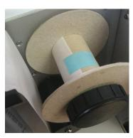
Before starting an aerosol sampling use the cycle "Insert filter" to wrap the filter tape a few times around the coil. This procedure shows whether the tape runs correctly through the stepper drive or not. Finally, the front hatch can be closed.
