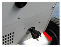
will disconnect the entire electronics. Then, the display switches completely off. After connecting the power supply it takes a few minutes to reach the battery voltage threshold which is required to turn on the unit again. The charging process takes about two hours and is indicated by the red light right beside the buttons. If the charging has been completed, the light turns off.
