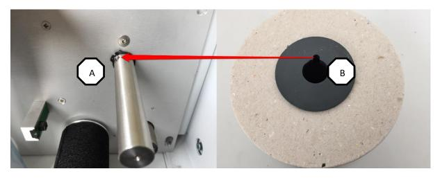
Attach the lock screws again after inserting the fresh filter coil too. Make sure that the fresh filter coil can be turned without strain.
