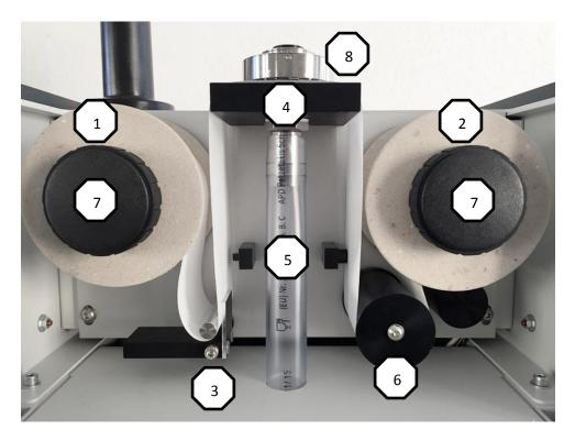
Stepper unit of standard version with open face air inlet
